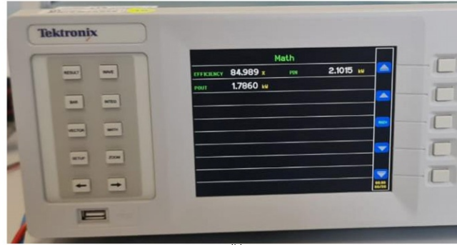
Fig. 8. Experimental results (a) Input 400 Hz voltage and current ( v_1 , i_1 ) and output dc side voltage and current ( v_{dc} and i_{dc} ) (b) the input and output power measured by the power analyzer.
