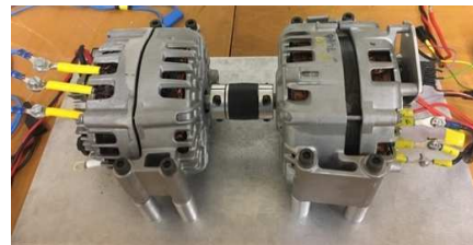
Fig. 1. Experimental test bench with two synchronous claw-pole machine
